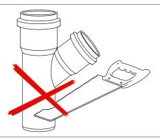
Do not shorten the fitting spigots, this would compromise the required insertion depth and the guarantee of a watertight seal.
