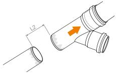
4) Insert the fitting onto the end of the pipeline to maximum socket depth and measure the resulting distance L2.
