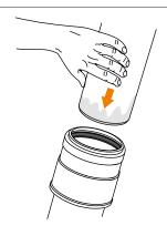
8) Make the joint by inserting the pipe inside the bi-joint.
