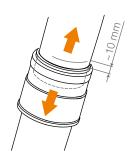
10) Pull back the spigot about 10 mm, this length allows any thermal expansion to be accommodated. If the spigot is that of a fitting then this operation is not required. Attention: do not pull back more than 10 mm as the seal of the joint would not be guaranteed or it could generate an excessive misalignment; if the spigot is pulled back less than 10 mm then the correct compensation of the thermal expansion would be prevented.
