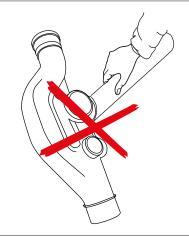
8) During this phase, avoid rotation or bending. It is possible to use a guide to keep the parts aligned during the welding process
