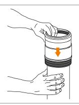
5) Fit the bi-joint onto the pipe where the grommet has been placed until maximum socket depth and check that the grommet is positioned correctly.
