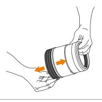
2) Inspect the condition of the bi-joint, clean the ends and remove the rubber grommet.
