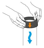
3) Fit the rubber grommet onto the pipe to be connected. The pipe onto which the grommet is fitted does not need to be chamfered. Attention: the position of the rubber grommet also defines the direction of the flow of the waste water.
