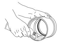
4) Spread both of the internal ends of the bi-joint with suitable Valsir lubricant (do not use mineral oils or grease).
