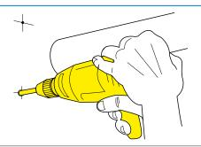
5) Drill the holes for the wall plugs and clean the holes of any debris. To fasten use Fischer FZA 10x40 M 6/10 or FAZ II 8/10 plugs that are suitable both for compact and cellular concrete.
